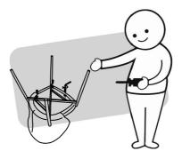
Unless instructed, do not fully tighten screws until the item is fully assembly.
